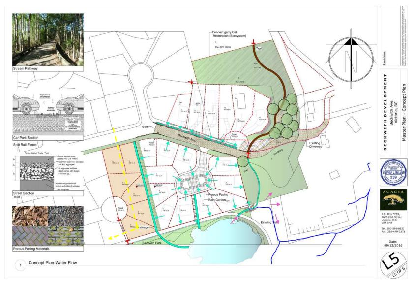
Conceptual routing of rainwater runoff from the three property parcels. Note the existing drainage from Beckwith Avenue drains south as shown by the dashed yellow arrows. The proposed re-routing of the runoff would be into Beckwith Pond, shown by the solid green line.
